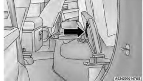
**Load Floor Securing Straps/Crew Cab**
