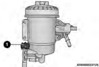
**Engine Mounted Fuel Filter Assembly**
