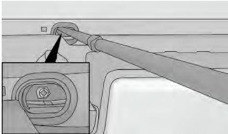
**Winch Mechanism Tube**
