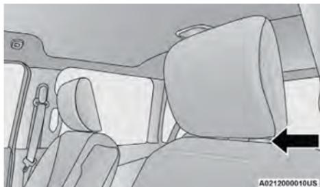
**Head Restraint Adjustment Button Location**
